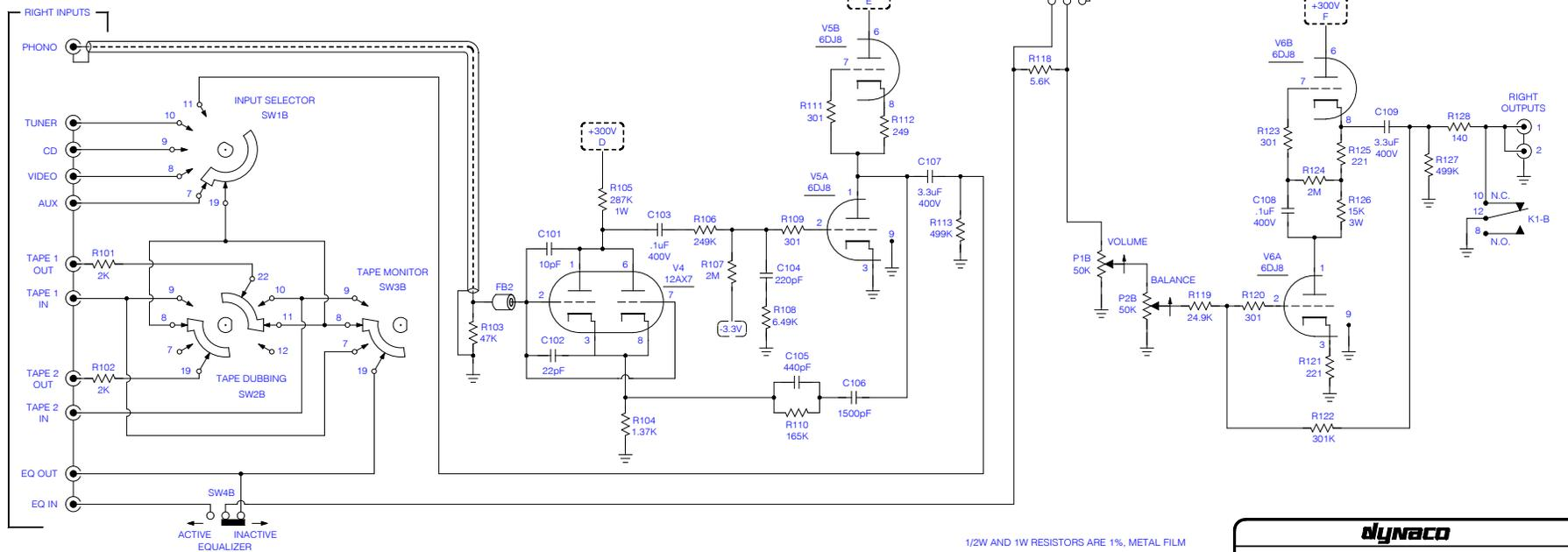
1/2W AND 1W RESISTORS ARE 1%, METAL FILM
